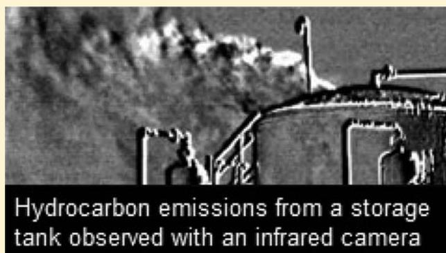
Hydrocarbon emissions from a storage tank observed with an infrared camera
