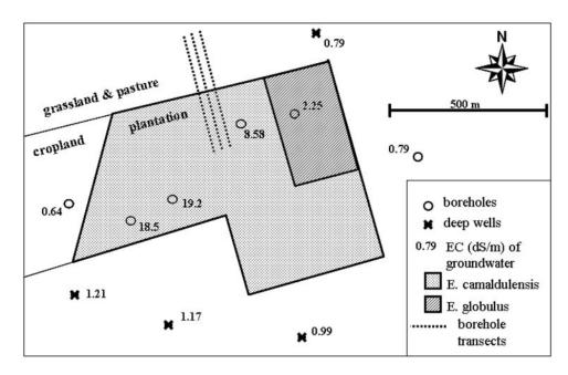
**Figure 2.** Diagram of the study site at Castelli. Ground water was sampled at the water table in 45 boreholes along the dotted transects and additional locations. Electrical conductivity (EC) values (dS/m) at the water table level are shown.
